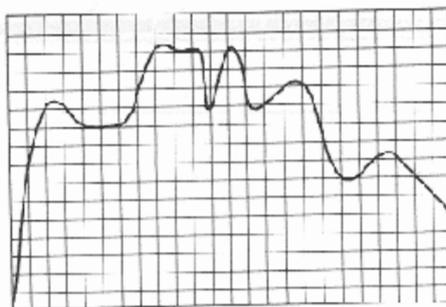
*Fig. 1c. DAC output filtered by ideal low pass filter.*
