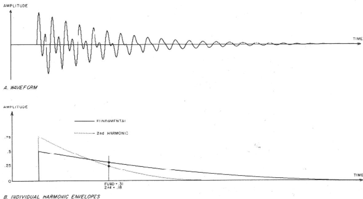
Fig. 2. Simplified characteristics of a plucked string.
