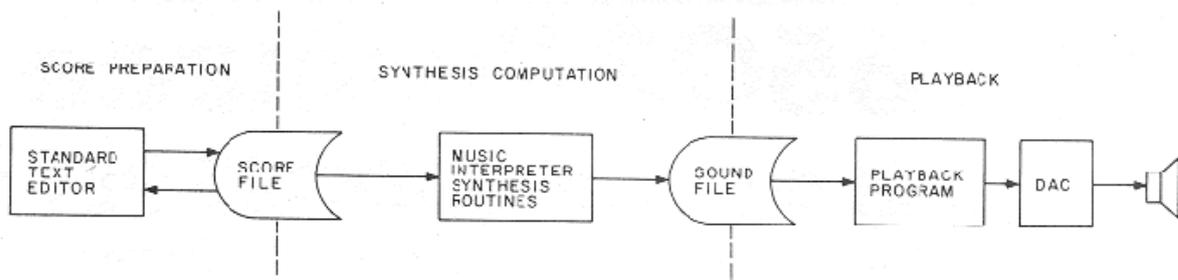
Fig. 4. Delayed-playback software synthesis system.
