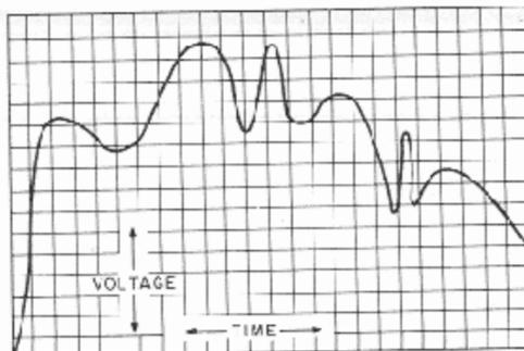
*Fig. 1a. Desired audio waveform.*
