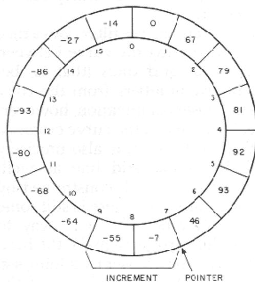
Fig. 4. Waveform table scanning.
